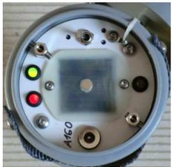
Charge current is limited by the max. output current of the solar module (420mA) and also by a fuse which automatically interrupts charging with too high current. The integrated control system avoids too frequent charging. **The lower limit voltage** is indicated by **a red warning LED**.
