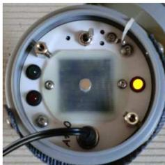
An automatic cut off of the loading current is not part of the design due to the low current of the solar module of 420 mA. There is no danger of overloading the NH batteries.
